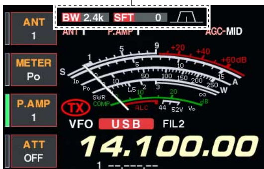
Shows filter width, shifting value and condition
